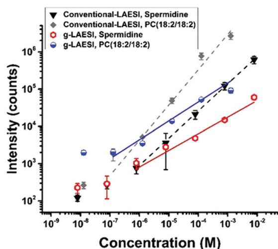
Fig. 5 Comparison of analytical figures for gradient and conventional LAESI-MS. Using g-LAESI, a limit of detection (LOD) of 79 and 13 fmol were obtained for spermidine (red hexagon) and PC(18:2/18:2) (blue circle), respectively. Same LODs were achieved for these two analytes using conventional LAESI (spermidine: black triangle, PC(18:2/18:2): gray diamond). Over four orders of magnitude dynamic ranges were observed for both gradient and conventional LAESI-MS.
