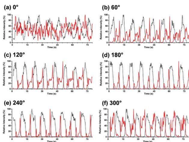
Fig. 3 Ion chromatograms for two spray solutions, 0.1  $\mu\text{M}$  verapamil in 2:1 (v/v) acidified methanol/chloroform (red solid line), and 0.7  $\mu\text{M}$  arginine in 1:1 (v/v) acidified acetonitrile/water (black dotted line), with two triangular high voltage waveforms (0.1 Hz frequency, 800 V amplitude, and 850 V offset) supplied at voltage phase differences of (a)  $0^\circ$ ; (b)  $60^\circ$ ; (c)  $120^\circ$ ; (d)  $180^\circ$ ; (e)  $240^\circ$ ; and (f)  $300^\circ$ .
