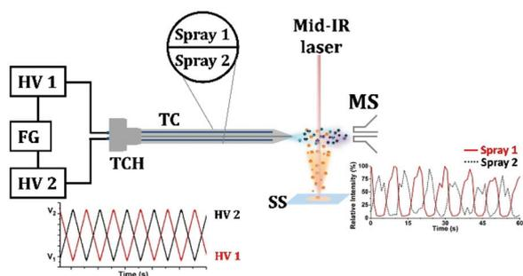
**Fig. 1** Schematic of gradient LAESI (g-LAESI). FG: dual-channel function generator, HV 1 and HV 2: high voltage power supplies, TC: theta glass capillary, TCH: theta glass capillary holder, SS: sample stage, MS: mass spectrometer.
