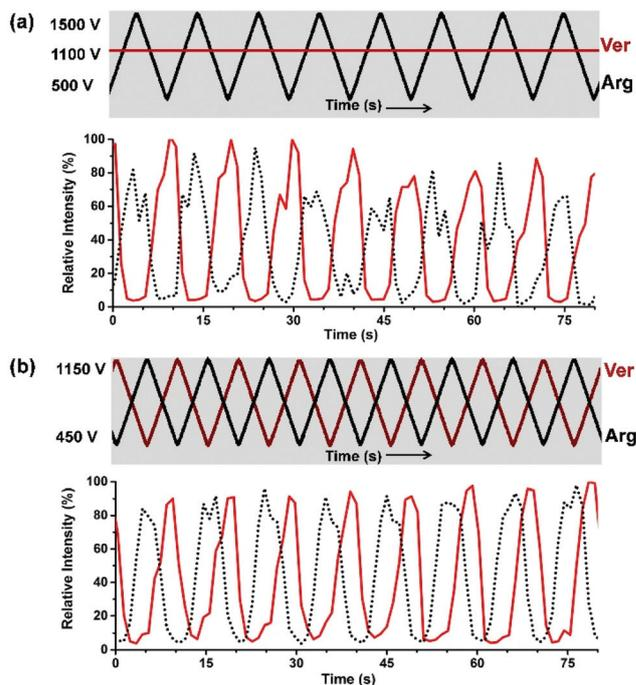
**Fig. 2** Ion chromatograms for two sprays and corresponding high voltage waveforms with (a) one constant and one triangular pattern, and (b) two triangular patterns. Time dependence of relative ion intensities for arginine (black dotted line), and verapamil (red solid line) exhibited periodic behavior that followed the periodicity of the high voltage.
