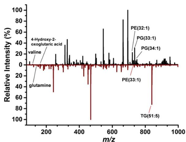
**Fig. 7** g-LAESI mass spectra of *E. coli* cell pellets acquired in two different phases of the gradient electrospray (10 to 15 scans each) produced from 1:1 (v/v) acidified methanol/water (top trace), and 10:7:3 (v/v/v) acetonitrile/methanol/toluene (bottom trace).
